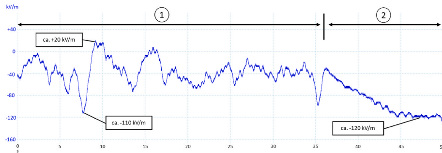
Fig. 13. Measured values of the electric field strength of the material web during machine startup and acceleration in the area after the unwinder.
